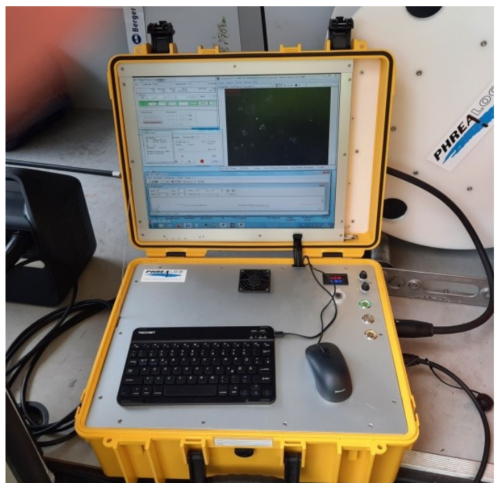
Field computer for analyzing the image data
