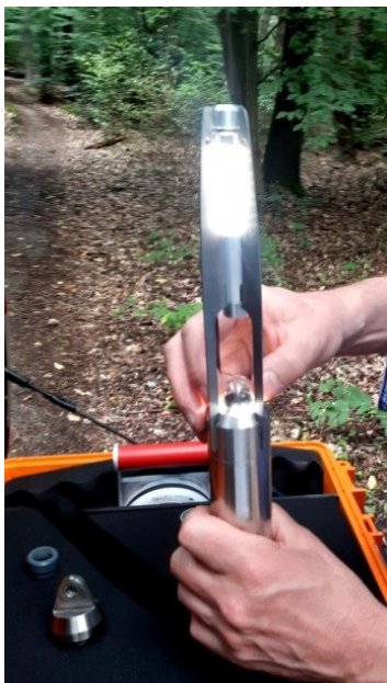
Auxiliary light head for wells exceeding 10 inches (DN250)
